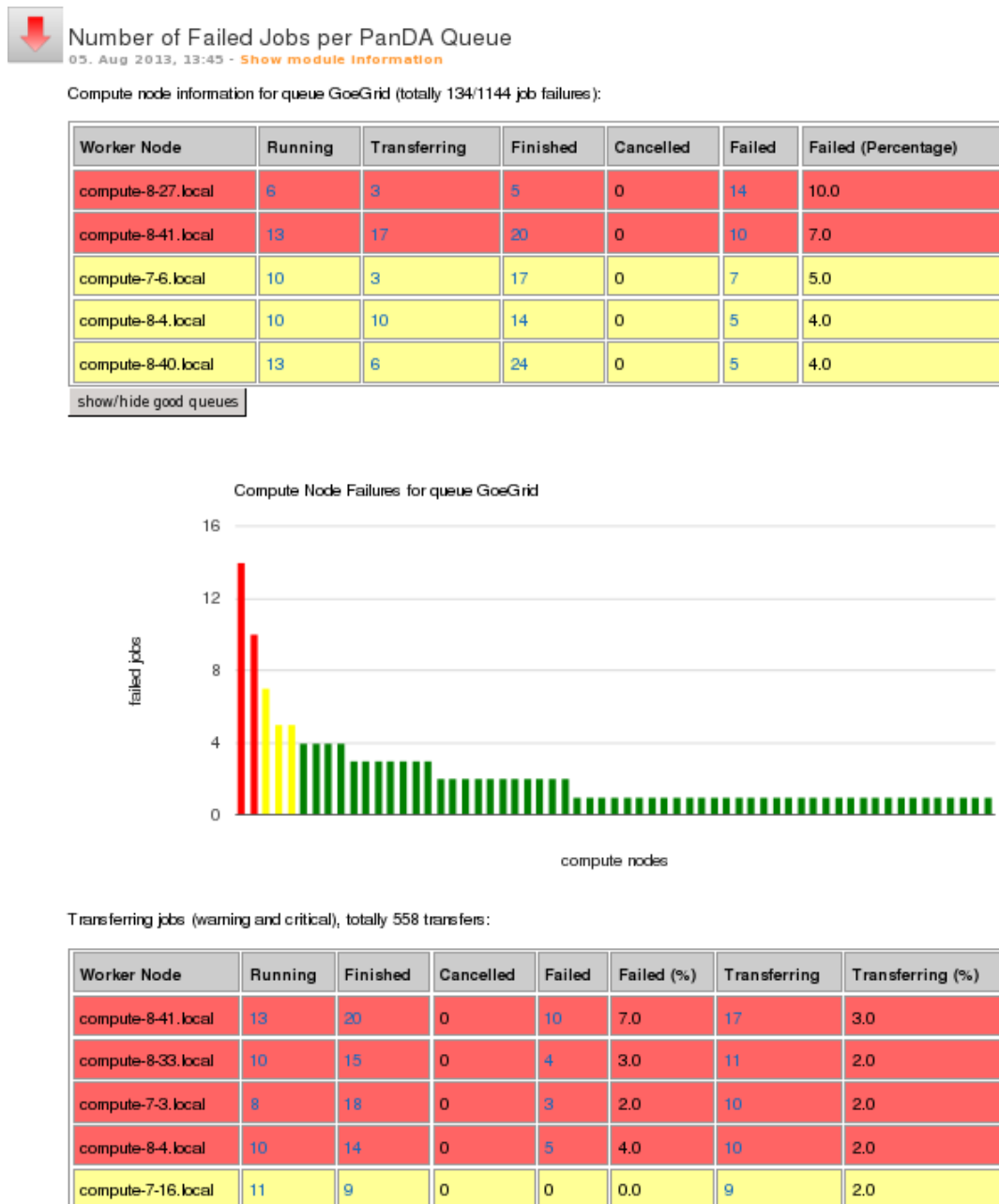
Figure 5.3.: View of the compute node information module in production for GoeGrid. The module contains two tables and one bar graph for each PanDA queue specified in the module configuration file.
