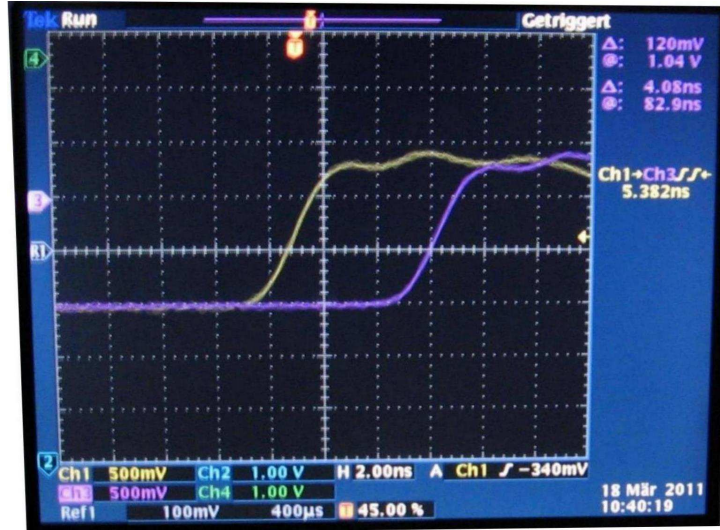
Figure 6.4: Example of a cable delay time measurement for a 5 ns delay LEMO cable.
