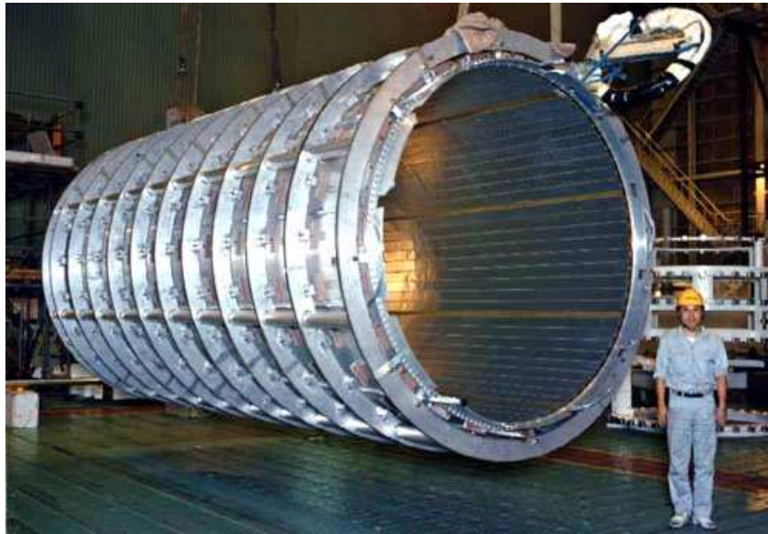
Figure 2.6: The ATLAS solenoid magnet [10].
