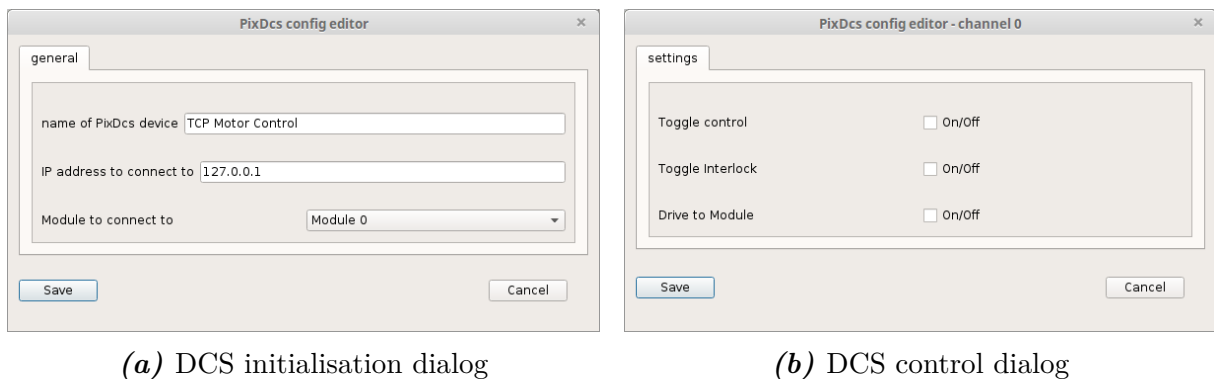
Figure 4.15.: DCS interface of the TCP control mode in STcontrol.
