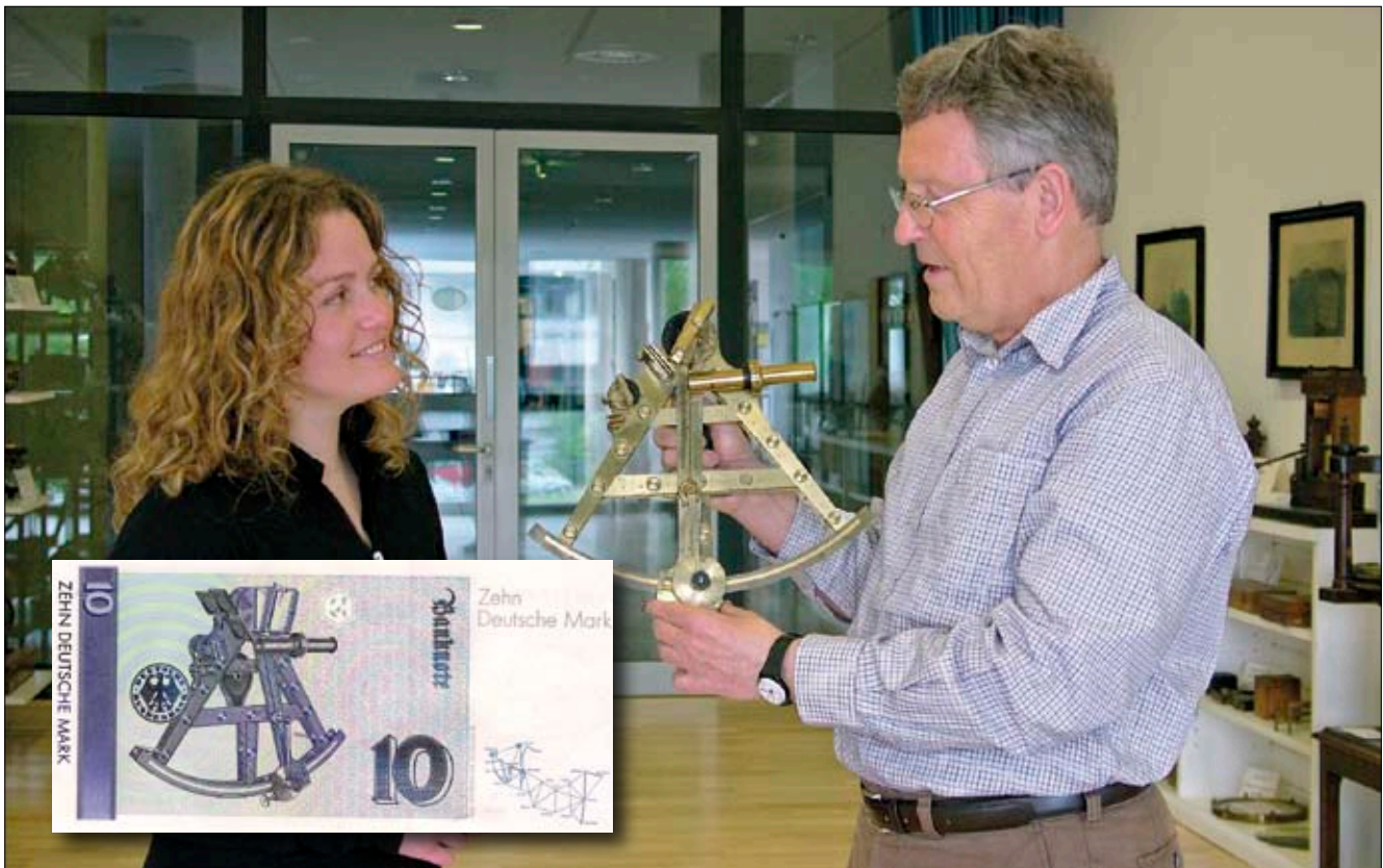
Fig. 4: Gauß's Vize-Heliotrop (manufactured by Troughton, London, 1810) in the hands of Prof. Gustav Beuermann. It was on the back of the 10 DM note. It was developed for a measurement campaign in the kingdom of Hanover, and its sensitivity allowed the study of the spherical access of the curved earth's surface.
