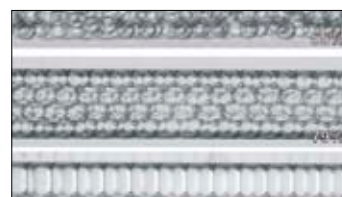
Fig. 1: An emulsion of equally sized water droplets in oil. As the droplets are pumped past the corner, well-defined changes in their relative arrangement occur. This may be used for 'chemical micro-processors', or other sophisticated micro-fluidic devices.
