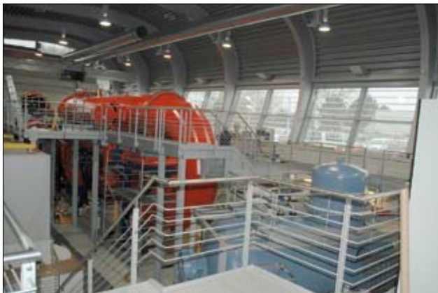
Fig. 1: Göttingen Turbulence Facility. The red tunnel is 18 m long and 6 m high. The blue 'Uboot' has a 2.5 m diameter and is 5 m long, the turret is 4 m high. The vessels can be filled up to 20 bar with SF 6 gas.
