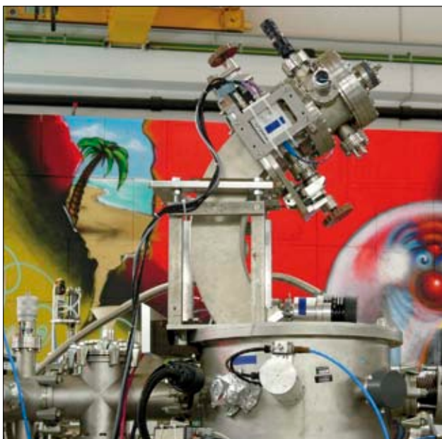
Fig. 1: High resolution RBS setup showing the scattering chamber and the cylindrical electrostatic analyzer providing a depth resolution of < 2 nm (Wallpainting by Helge Steinmann).
