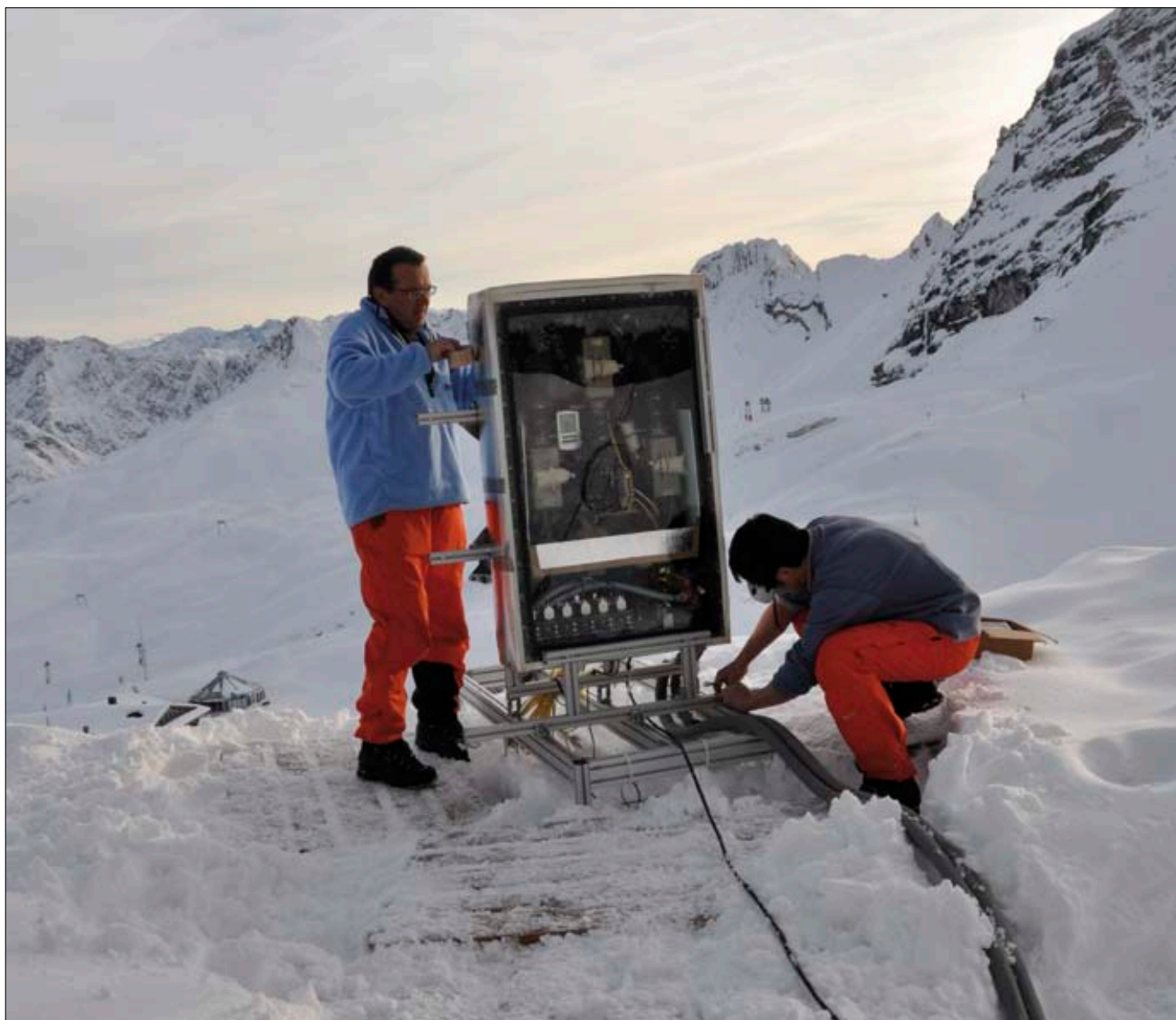
Fig. 2: 3D droplet imaging system being installed at Environmental Research Station Schneefernerhaus at 2700 m.
