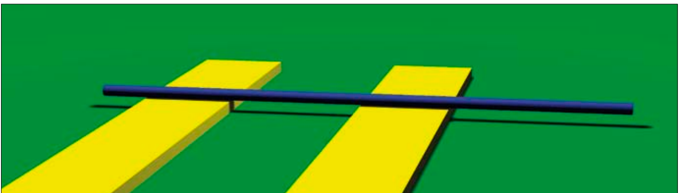
Fig. 1: Sketch of a typical experimental setup used to study the conductance of quantum wires. The wire is attached to higher dimensional leads, which further extend outside the image.
