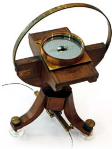
Fig. 6: Weber's instruments to measure the magnetic field generated by the circular current loop from 1837. With the Tangtenbussole (Bussole=compass), sensitive deviations of the needle were determined thus it was the first practical instrument to measure the magnetic field generated by the current through the wire loop. The wiring can be seen at the bottom.
