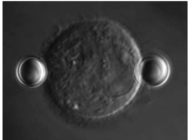
Fig. 7: Fibroblast cell suspended between two optically trapped beads of 4 micrometer diameter.
