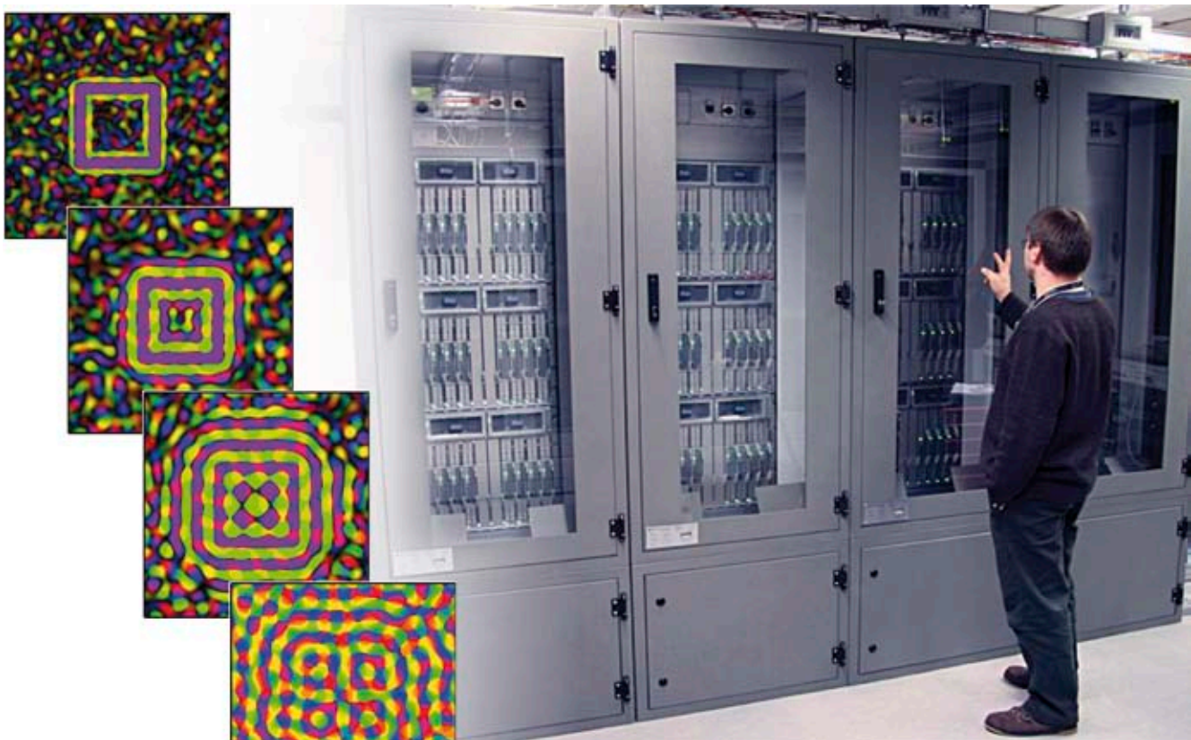
Fig 3: The Institute of Nonlinear Dynamics disposes of a set of dedicated high performance computing platforms, including the cluster of blade servers with 640 CPU cores shown above. They are used e.g. for simulation studies of the dynamics of neuronal activity in brain models, calculations of quantum mechanical wave propagation in complex semiconductor geometries, or studies of the dispersal of pathogens in human populations. The panels on the left show snapshots from a simulation of self-organizing neuronal circuits in the visual cortex of the brain. Colors encode the angle of preferred visual stimuli. In this simulation, the network was prepared by external stimulation in an initial state of approximate square symmetry. The state dynamically decays into a complex pattern, retaining signatures of the square symmetry. The simulated region represents roughly 100 million neurons.
